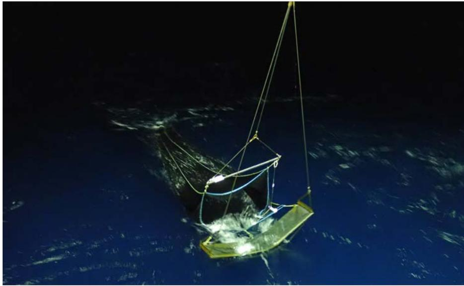
Figure 8. The Isaacs Kidd Midwater Trawl being recovered. Wire-out speeds were 10 – 30 meters per second, and haul-back speeds were 10 to 30 meters per second. Tow depths ranged from 300 m to 1200 m. Photo credit: Joe Warren
