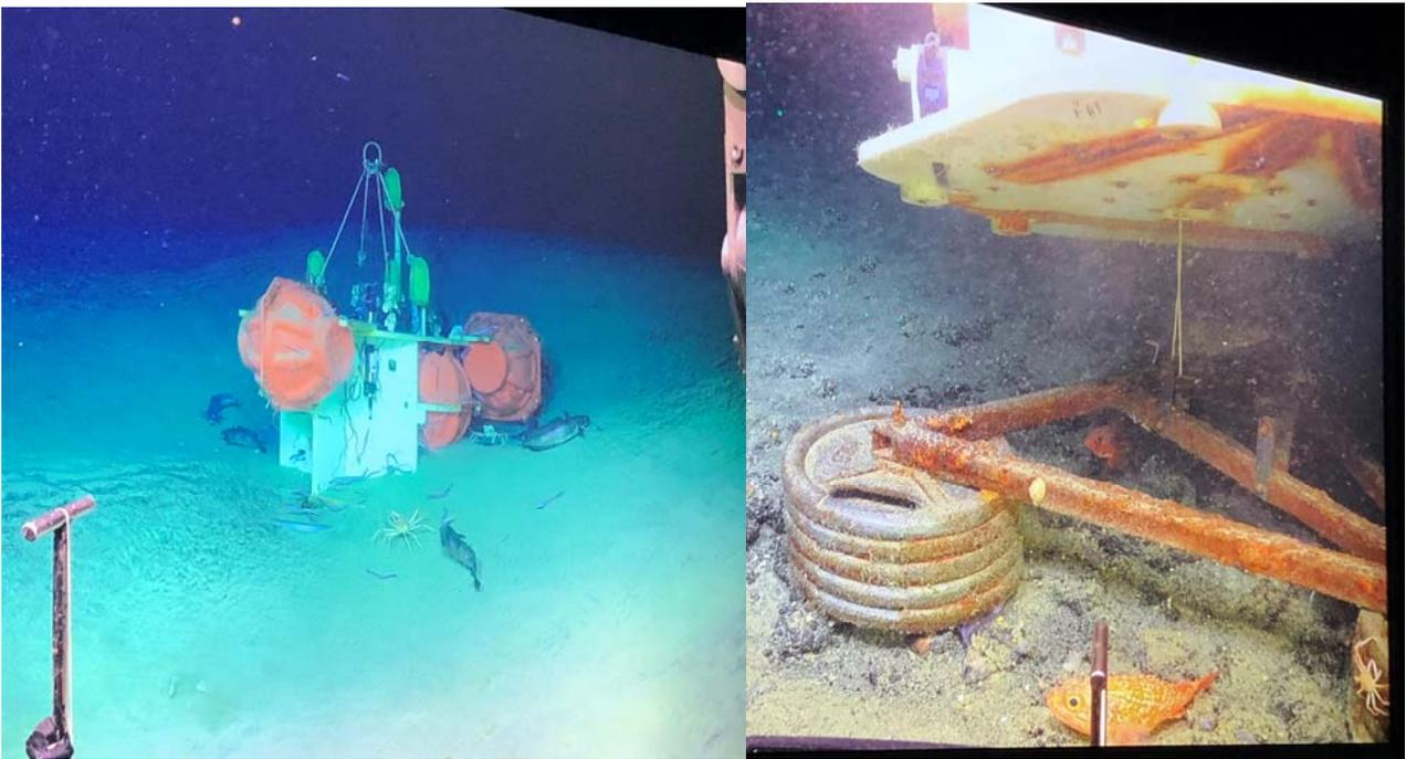
Figure 16. Left – ADEON WIL lander buried in sediment which prevented surfacing despite successful release. Right – ADEON JAX 2018 lander showing caught release line that prevented surfacing. Both photos taken from cameras mounted on ROV Jason (Photo credit: Jennifer Miksis-Olds).
