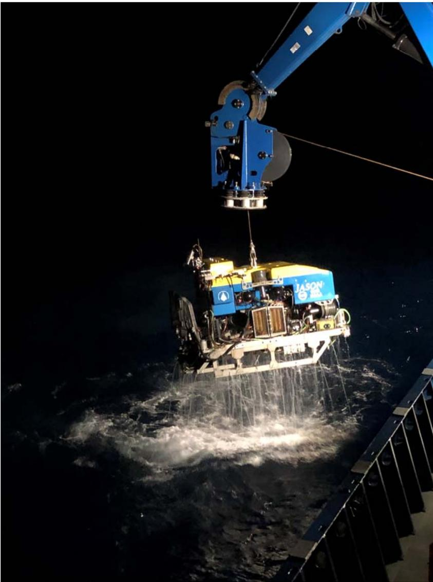
*Figure 17. ROV Jason returning to the deck of the R/V Armstrong after its final engineering dive to 3000 m . (Photo credit: Jennifer Miksis-Olds)*
