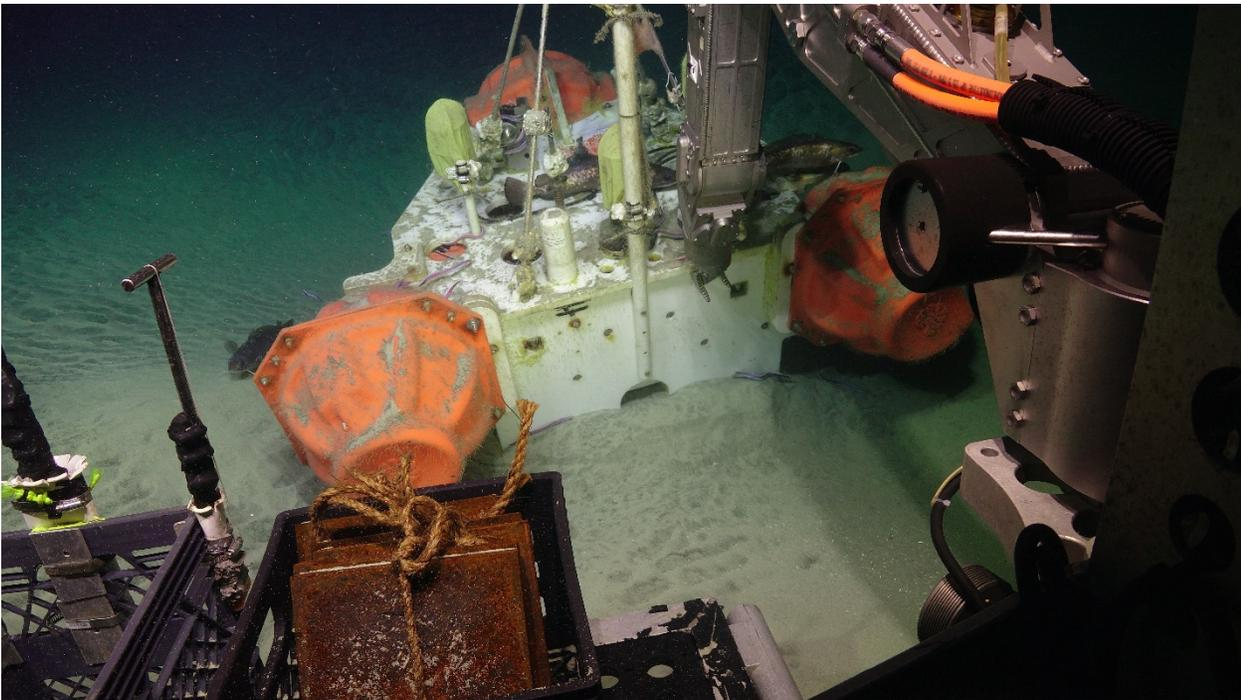
*Figure 3. Image captured from the ROV Jason cameras. The manipulator arm is prying the buried WIL lander from the sediment. (Photo credit: ROV Jason footage provided to Jennifer Miksis-Olds)*
