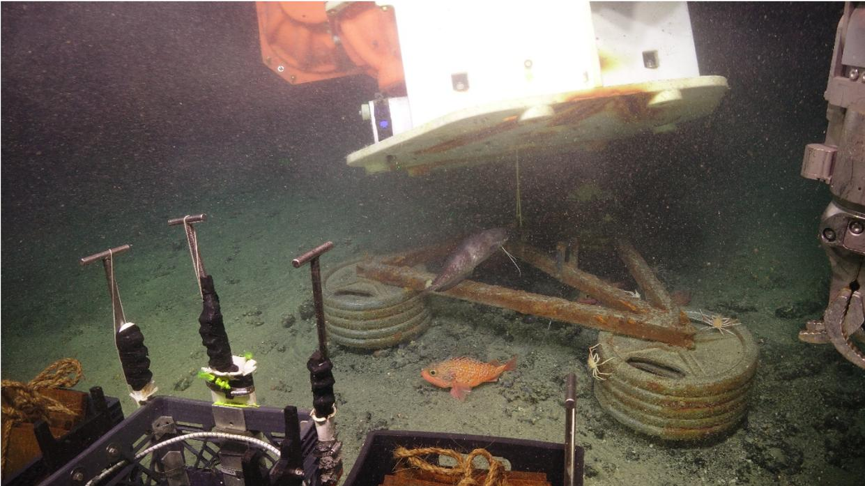
*Figure 4. Image captured from the ROV Jason cameras. The JAX lander released but the release line got caught up in the lander structure preventing it from surfacing. (Photo credit: ROV Jason footage provided to Jennifer Miksis-Olds)*
