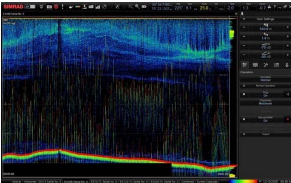
Figure 5. Example echograms from the ship's EK80 showing epipelagic scattering layers (top) as well as internal waves (bottom) which were commonly observed during the cruise as the ship transited across the continental shelf. These data are from the WIL fine-scale acoustic survey.
