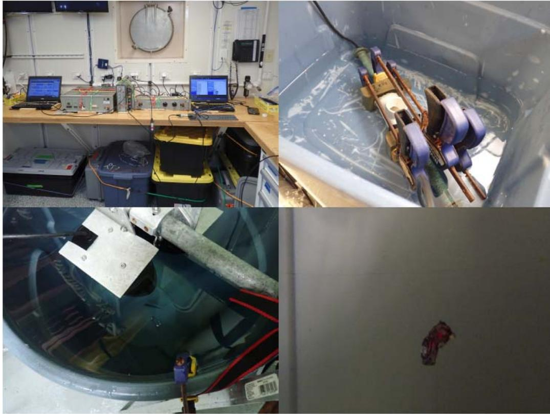
*Figure 11. All TS and  $h$  measurements were conducted in the wet lab using a power amplifier, match transformer, digitizing oscilloscope, signal generator, and a laptop (top-left). Sound speed contrast ( $h$ ) experiments were performed in a plastic bin so the brass 192 kHz transducers could remain submerged (top-right). TS measurements were made in a 44 gallon aquarium using urethane broadband transducers (bottom-left) on tethered animals such as the hatchetfish (bottom-right).*
