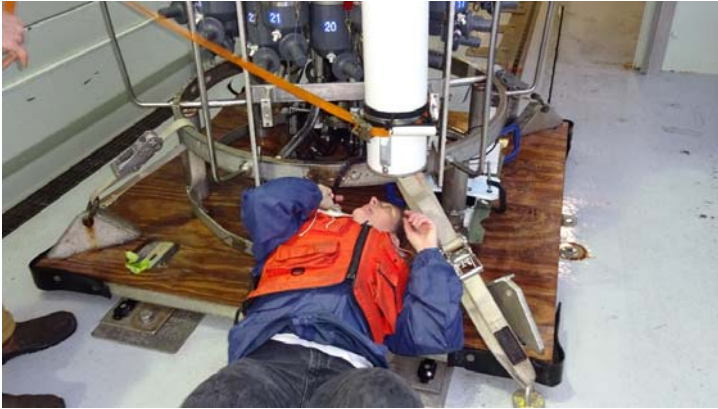
Figure 3. The AZFP transducers are being mounted to the bottom of the CTD frame by J. Miksis-Olds (left). AZFP transducers and battery pack mounted to the CTD frame (right).
