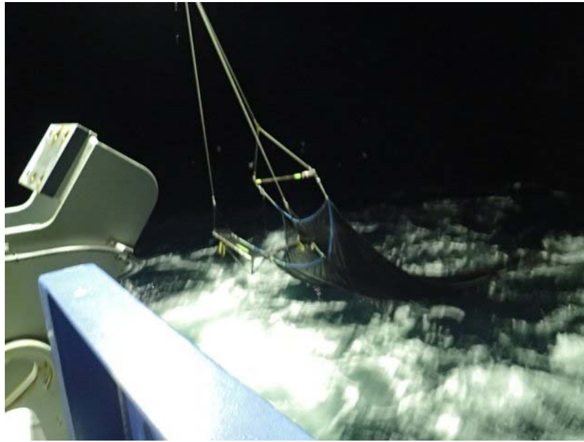
Figure 19. The Isaacs Kidd Midwater Trawl being deployed. Wire-out speeds were 20 – 40 meters per second, and haul-back speeds were 10 to 30 meters per second.
