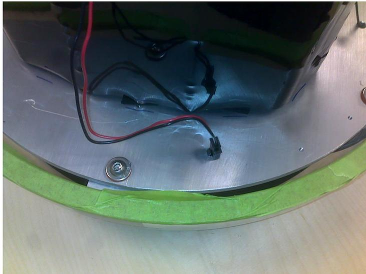
7. Place electronics hemisphere into hardhat temporarily to allow installation of the hydrophone and calibration.
