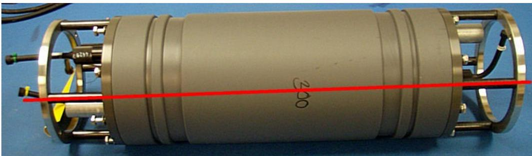
9. Install the bolts finger tight on the end cap.
