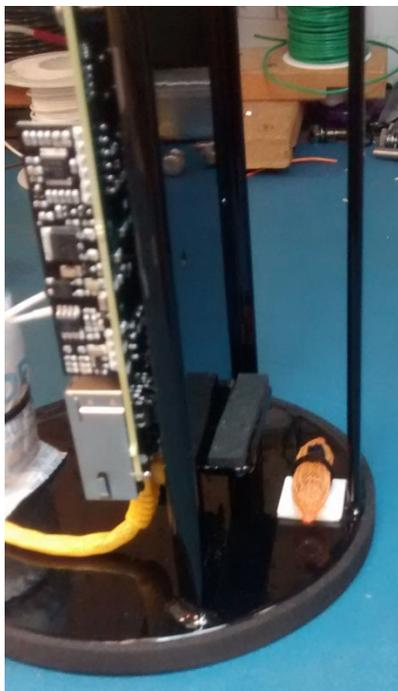
5. Insert top end cap into pressure housing, ensuring that no wires are pinched and that the battery, bolts/washers do not nick or damage the O-ring surface. Close the locking clamps.
