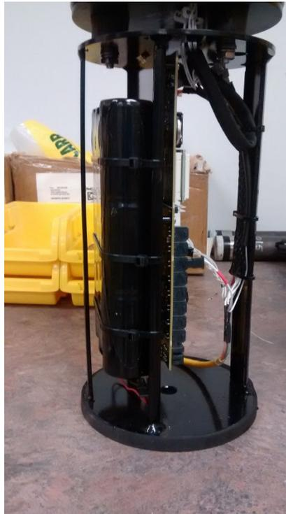
6. Insert top end cap into pressure housing, ensuring that no wires are pinched and that the battery, bolts/washers do not nick or damage the O-ring surface.
