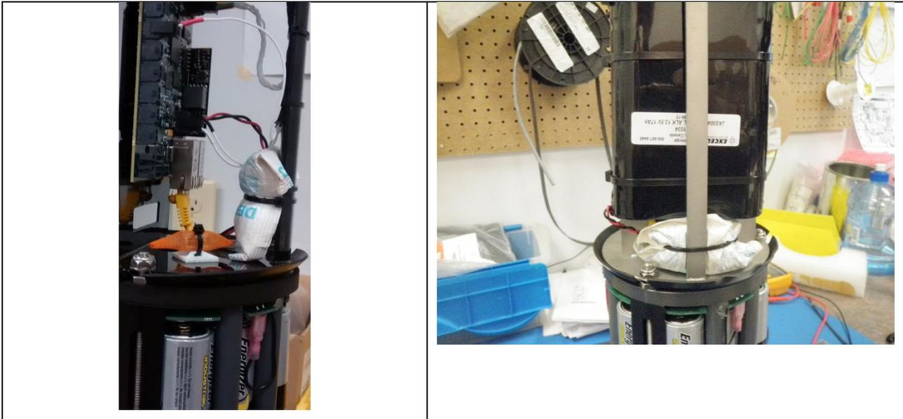
4. Verify hydrogen combiner pellets are installed and container is not damaged. Replace if required.
