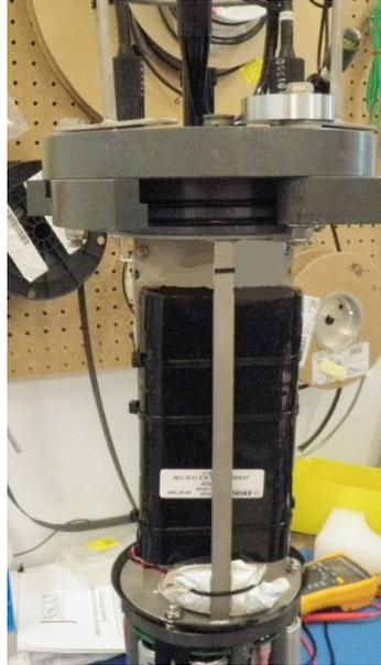
3. Verify that the total voltage across the battery pack at the power connector is at least 13.5 V and has the correct polarity. **Record** the voltage.
