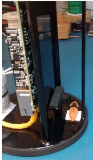
3. Insert top endcap into pressure housing, ensuring that no wires are pinched and that the bolts/washers do not nick or damage the O-ring surface.
