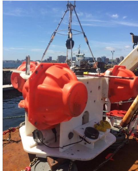
Figure 6. (Left) Bottom lander cut-away identifying the hardware components and (right) ADEON bottom lander on the deck of R/V Odyssey during trials in June 2017. Not shown in these images is a cylindrical flow shield around the M20 directional sensor to isolate it from flow.
