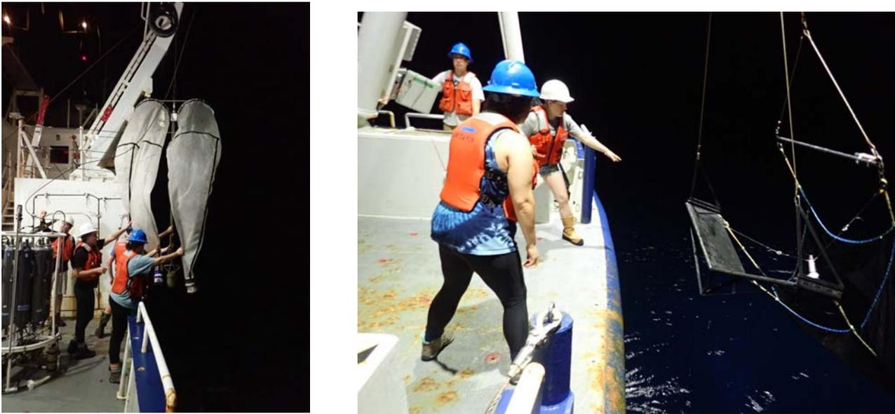
*Figure 9. Bongo net (left) being deployed for a vertical cast to a depth of 100 m. The Isaacs-Kidd Midwater Trawl (right) being deployed. Wire-out speeds were 20 – 40 meters per second, and haul-back speeds were 10 to 30 meters per second. Tow depths ranged from ~150 m to 1300 m. (Photos: Joseph Warren)*
