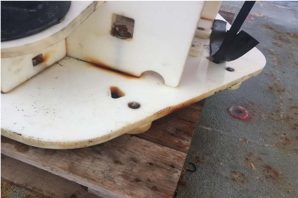
*Figure 4. Damage (scrapes on edges of lander) to VAC lander from possible trawl marks. (Photo: Carmen Lawrence)*
