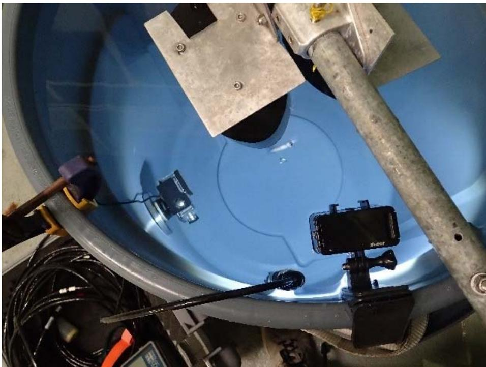
*Figure 11. Experimental aquaria set up of broadband transducers, underwater camera to monitor the orientation of the animals, LED lights to increase visibility, and a YSI 85 probe to collect real-time temperature and salinity data which affect the sound speed velocity in water. (Photo: Brandyn Lucca)*
