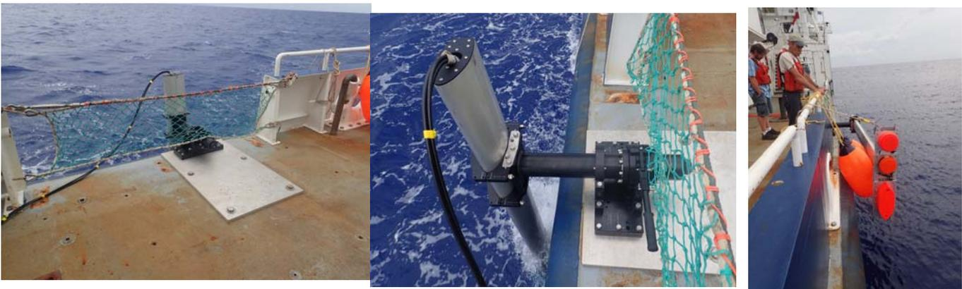
*Figure 7. To install the pole-mount system on the ship, a bulwark was removed, and a 4ft x ~2.5ft x 1” aluminum plate was bolted to the deck bolt grid. The pole-mount apparatus was attached to the aluminum plate with the pole in the horizontal position. (Photos: Joseph Warren from EN615 cruise)*
